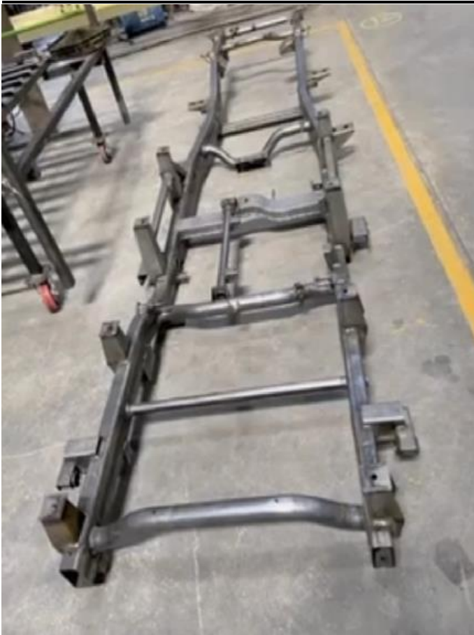
Fig 3.2: Final Structure of Chassis Line
