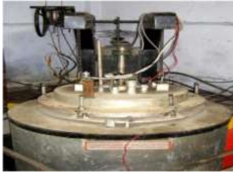
Fig. 1 Gas carburizing furnace
