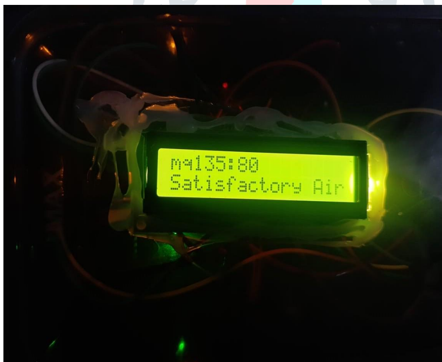
Fig 5:MQ-135 sensor reading on LCD when air quality is Satisfactory
