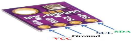
Fig 5. Pinout Cable BME280 Sensor
