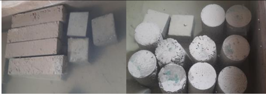
Figure 3. Curing of cubes, cylinder, beams
