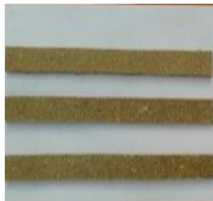
Figure 8: Flat Areca fibre and Glass fibre reinforced composite specimen used for Flexure testing.
