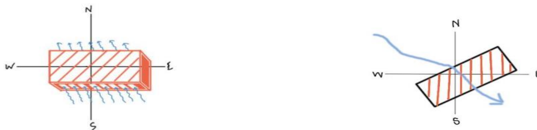
Figure 2 (left) Optimum orientation w.r.t to the sun direction and, (Right) Optimum Orientation as per wind direction
