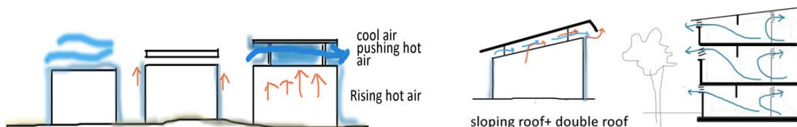
Figure 7 Different types of double roof techniques
