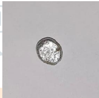
Fig. 6 Piece of Silver metal obtained after ignition
