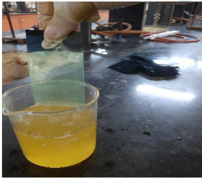
Fig. 5 Film dipped in 1M Nitric acid solution
