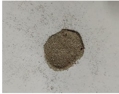
Fig. 4 Precipitated Silver dust
