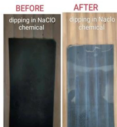
Fig. 3 X-ray films before and after dipping in solution
