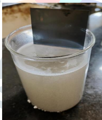
Fig. 2 X-ray films dipped in sodium hypochlorite solution
