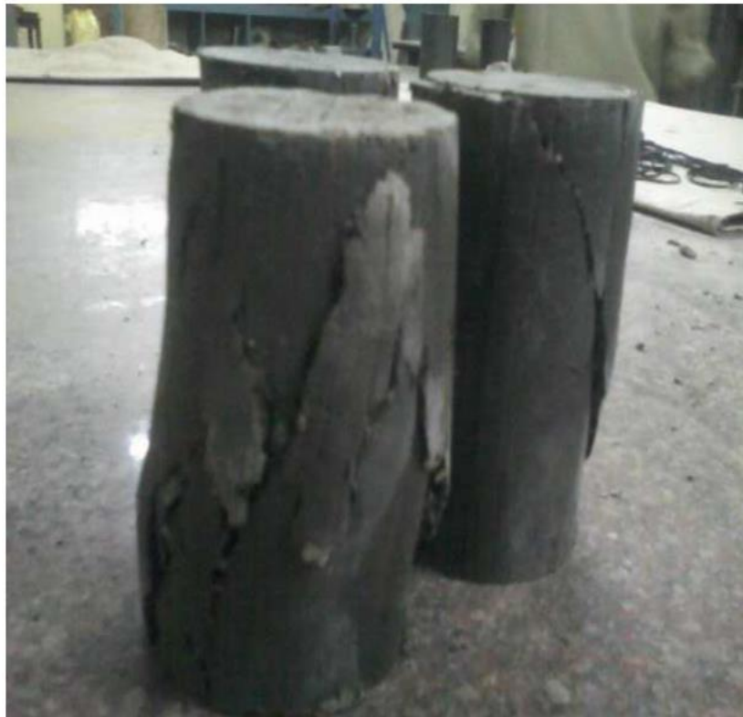
Fig. 3.2: Samples after failure at different confining pressures
