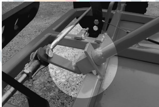
Figure 4.3 Assembly of Steering Shaft and Brackets
