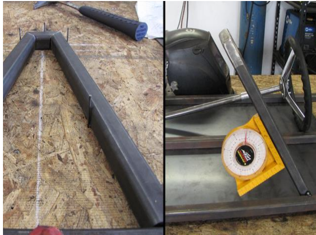
Figure 4.2 fabrication and assembly of Steering Hoop
