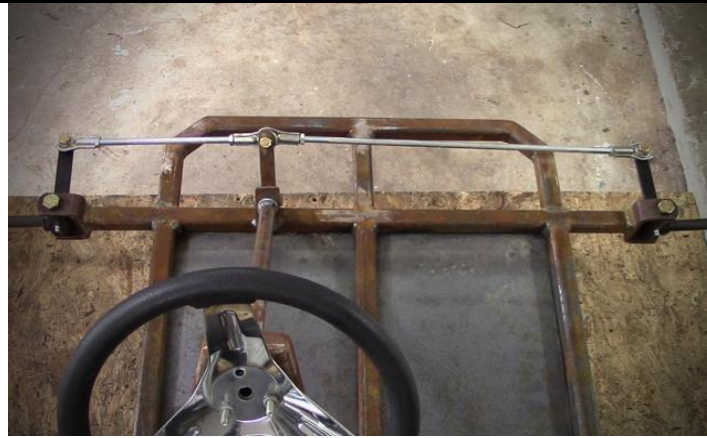
Figure 4.4 Assembly of Spindle brackets and Tie rods to front axle.
