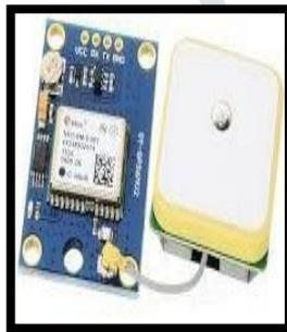
Figure 3: GPS Modem
