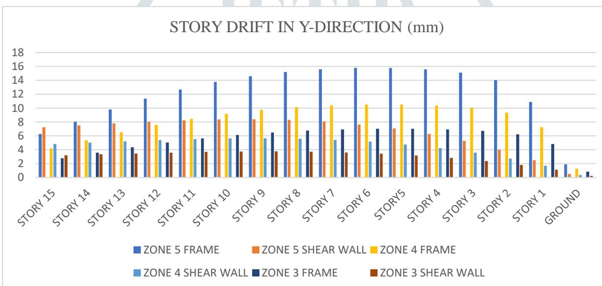
Fig 5.4 Storey Drift at Y-direction
