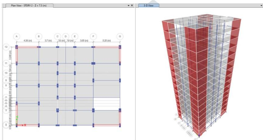
*Fig 4.2 Shear Wall Layout and Elevation of Shear Wall Structure*
