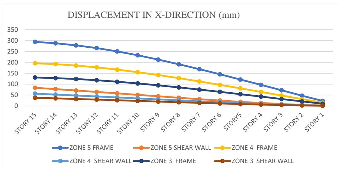
Fig 5.1 Displacements of X-direction
