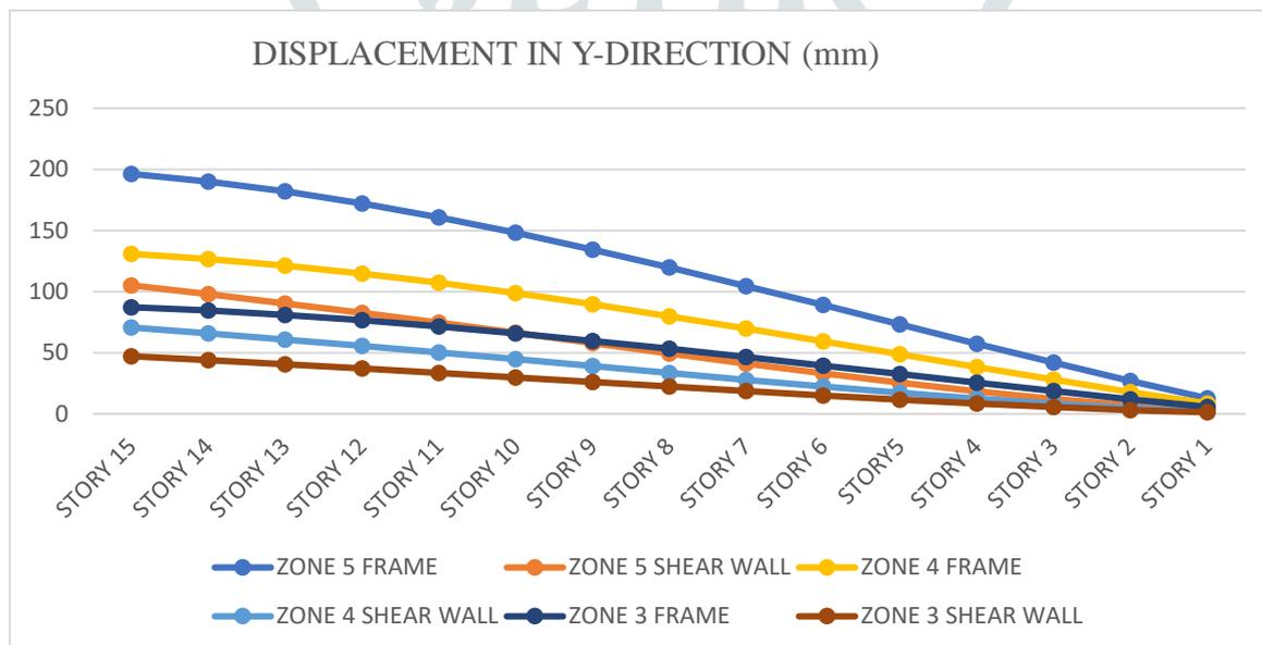
Fig 5.2 Displacements of Y-direction
