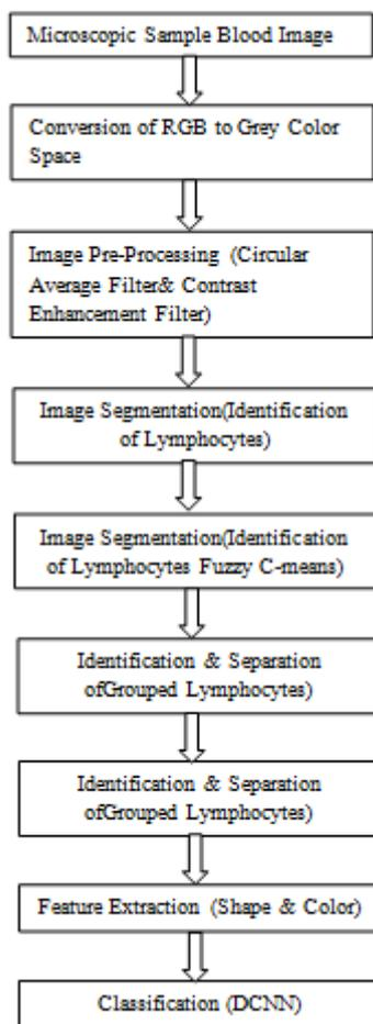
Fig.9: Proposed Block Diagram
