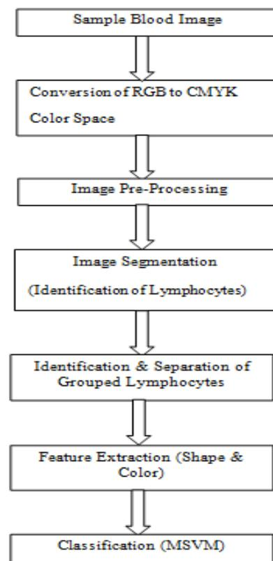
Fig.3:Existing System block diagram
