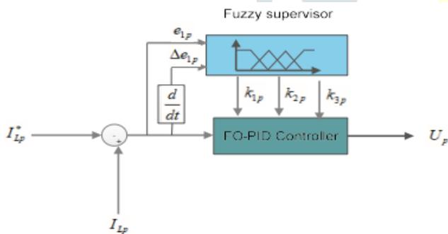
FIGURE 7. SSCs controller law computation with the IFO-PID
