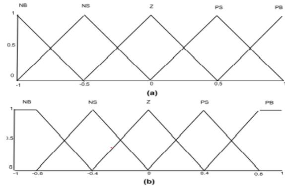
FIGURE 8. The fuzzy controller configuration. (a) Input membership function, (b) Output membership function
