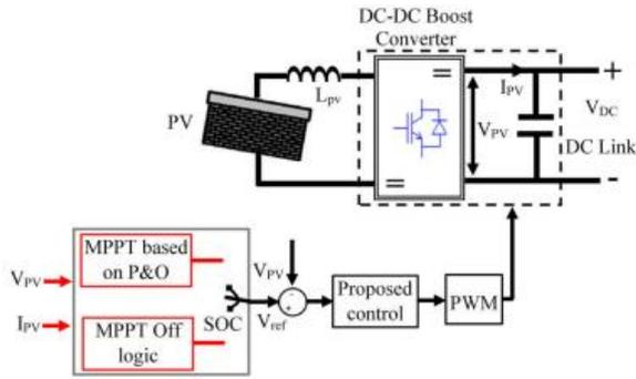
FIGURE 4. Solar energy system with controller
