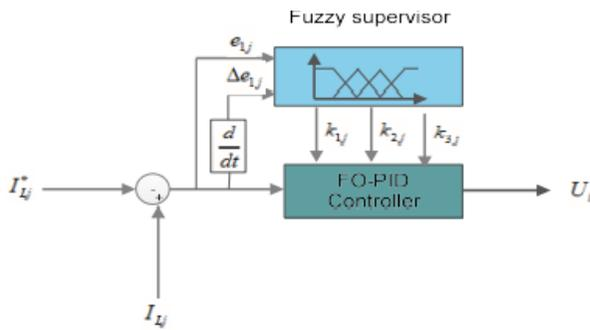
FIGURE 9. SSCs controller law computation with the IFO-PID.
