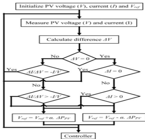
FIGURE 5. MPPT algorithm of the solar energy system.
