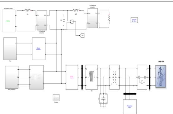
Figure 23: Simulink model grid connected Hybrid system
