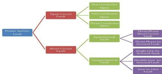
Figure 12: Different types of faults occurred in the system
