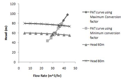
Fig.6 PAT Curves diagram between head and flow rate.
