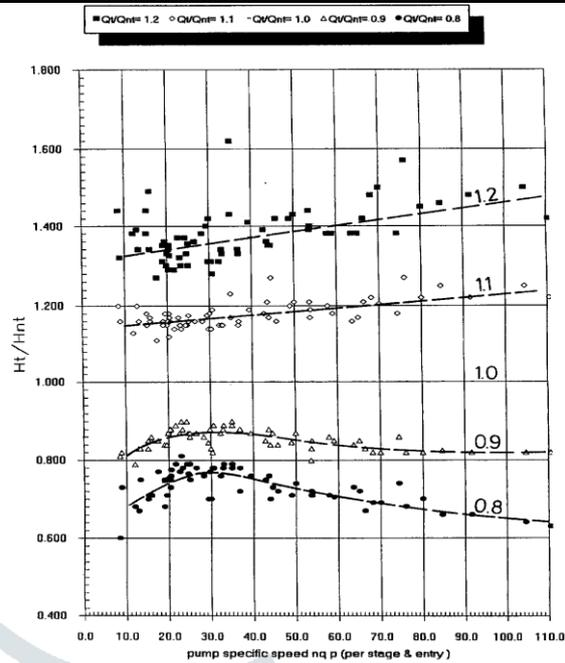
Fig.4 Turbine-Mode performance from the BEP
