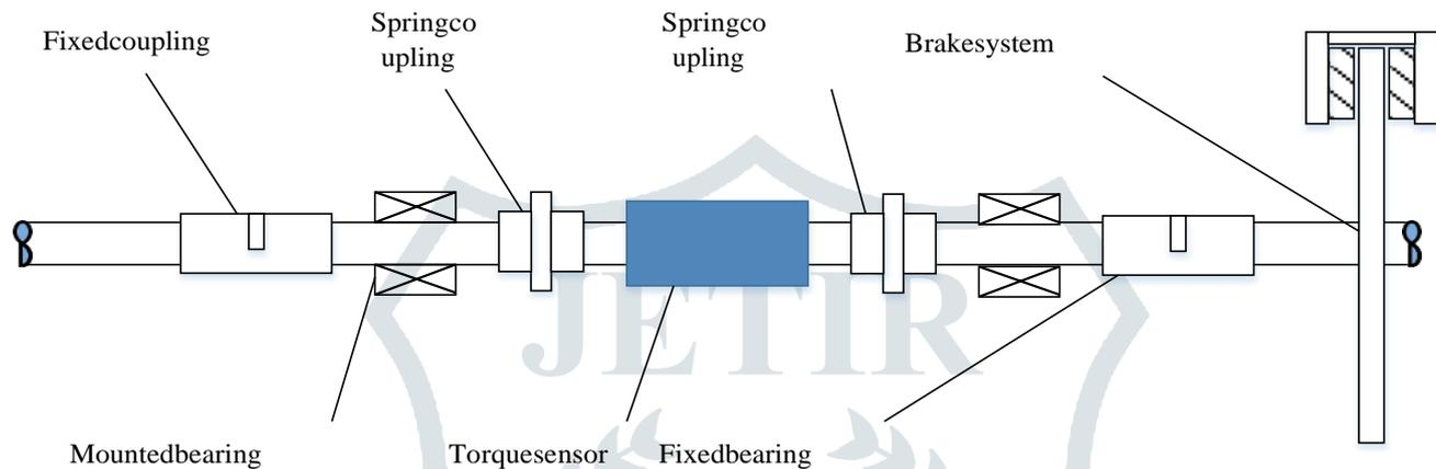
**Fig2. Schematic illustration of braking system using torque sensor and fittings**
