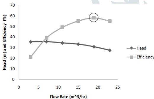
**Fig.5 Head v/s Flow rate and also ‘Efficiency v/s Flow rate’ curves.**
