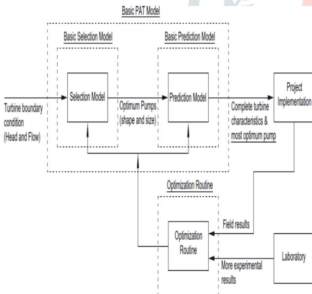
Fig.3 combined structure of pumps such as turbines with optimization routine are displayed below
