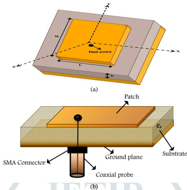
Fig. 1: Basic Configuration of microstrip antenna (a) Top view (b) Side view
