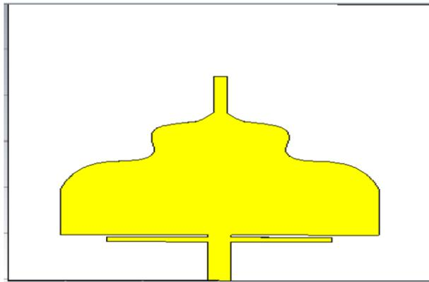
**Fig. 7: Parasol Design of Microstrip Antenna**
