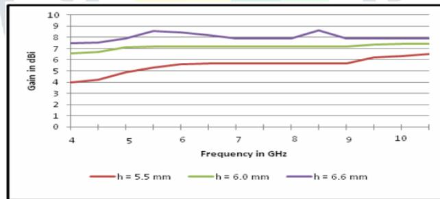
Fig. 5: Gain variations of microstrip antenna
