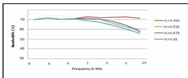
Fig. 6: Bandwidth variations of microstrip antenna
