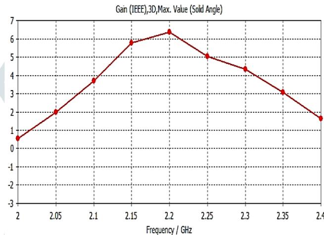
Fig. 11: Gain vs frequency plot
