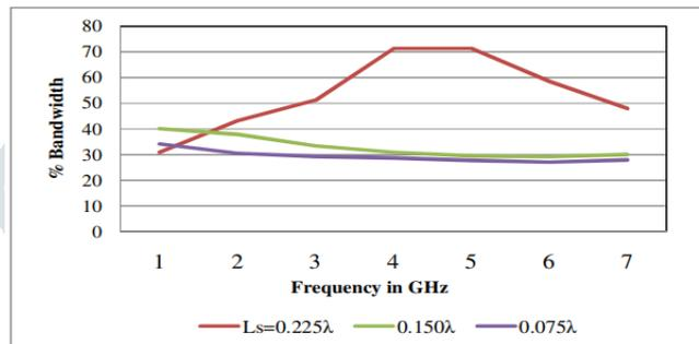
Fig. 4 Bandwidth variations for various slot lengths
