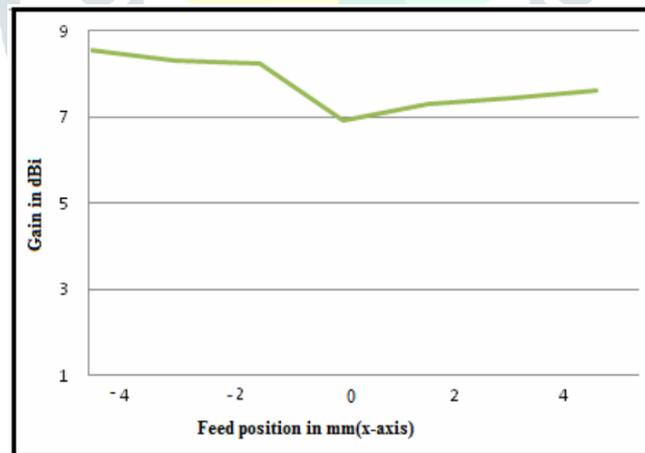
Fig. 2: Gain variations of microstrip antenna
