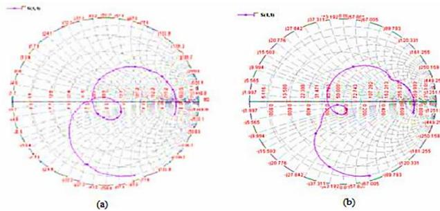
Fig. 3: (a) Smith chart for optimized gap width (b) Smith chart for increased gap width
