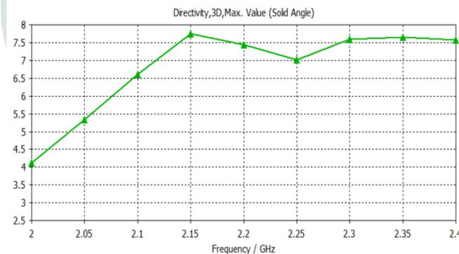
Fig. 12: Directivity vs frequency plot
