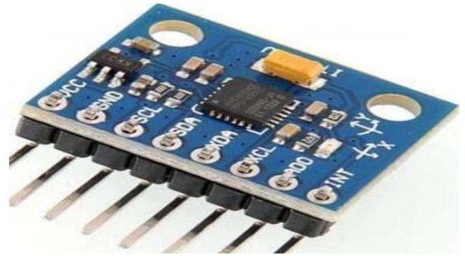
**Fig.6: Gyro Sensor**
