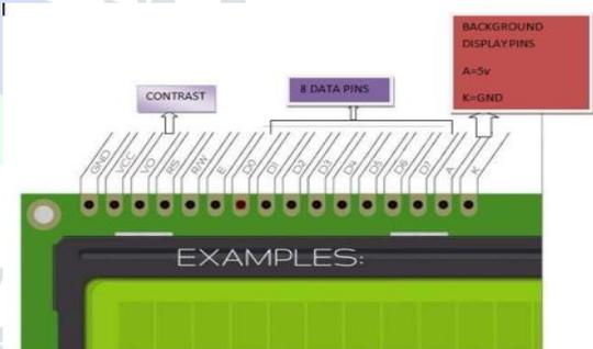
**Fig.7 16x2 LCD Display**
