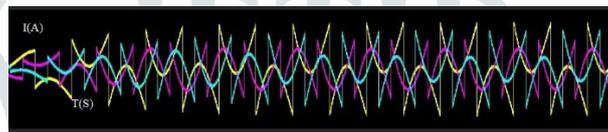
generated harmonics. These cancel out resulting in an acceptable level of harmonics. Compensating current waveform is shown in the waveform.
