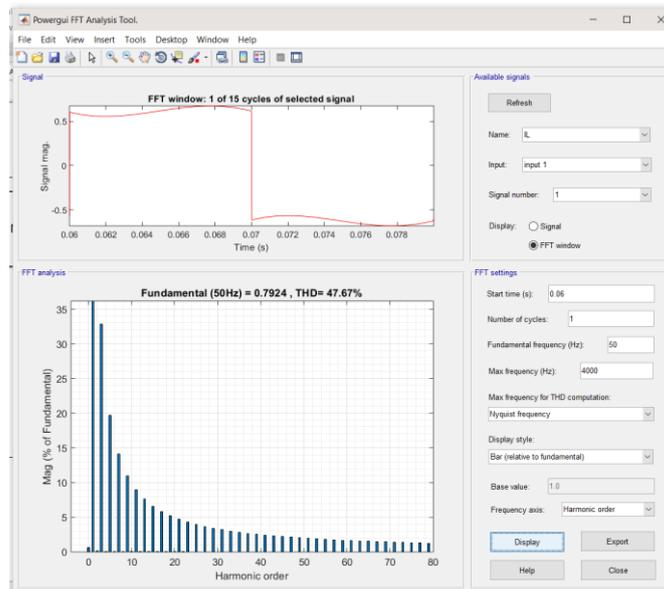
We can observe in above figure that the 47.67% of THD present in the load current
