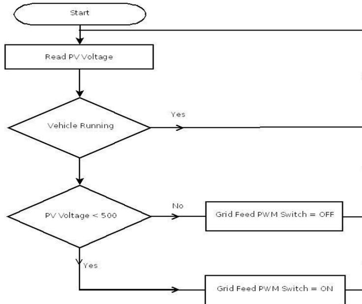
Fig.2: Flow Chart Of Photovoltaic Priority Battery Charging Using PWM Based Grid Subsidization.
