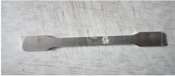
**Fig17: Frictionstirwelded partAl-Al**
