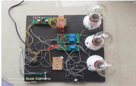
The output -1 is shown in the figure below when all of the nodes 1, 2, 3 are fault-free and all of the light bulbs are lit.
