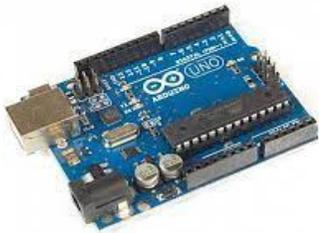
The ATmega328P microcontroller supports UART TTL (5V) serial communication via digital pins 0 (Rx) and 1 (Tx) (Tx). The serial communication is channelled over USB by an ATmega16U2 on the board, which appears as a virtual com port to software on the computer. The ATmega16U2 firmware relies on standard USB COM drivers and does not require an external driver. On Windows, however, an.inf file is required.
