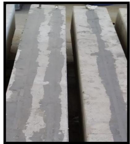
**Fig. 7 Filled Using Epoxy Adhesive**
