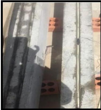
**Fig. 5 Grooving In Beam**
