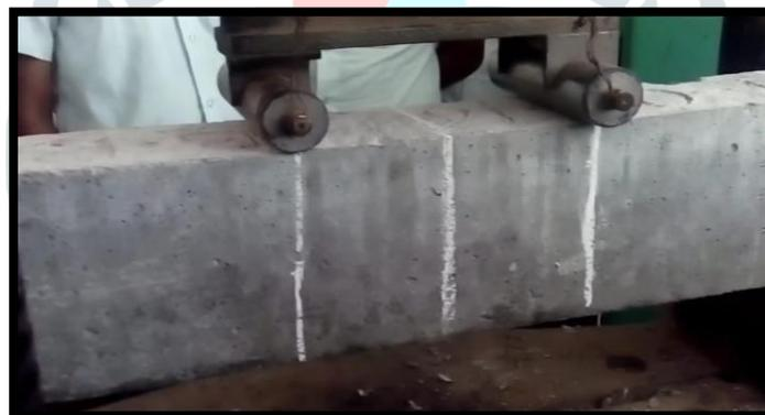
**Fig. 8 Testing Of Beam**
