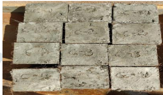
Fig 4.4 Demoulded bricks from the iron mould after one day
