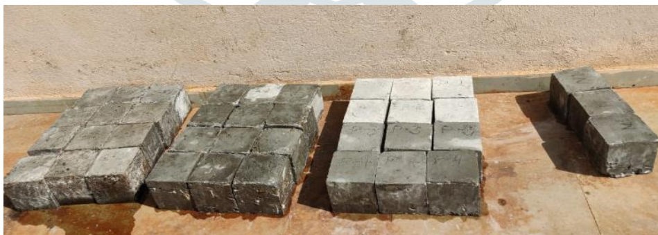
Fig 4.6 After 14 days of curing the bricks are removed from the water tank and kept for drying,
