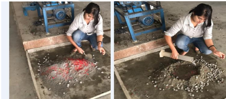
Fig 4.2 coir fibre,areca fibre,&amp; plastic waste with cement and other ingredients
