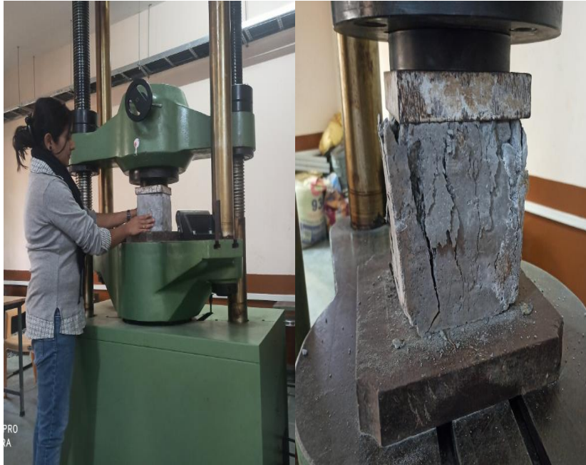
Fig 5.1 Testing of bricks for compressive strength
