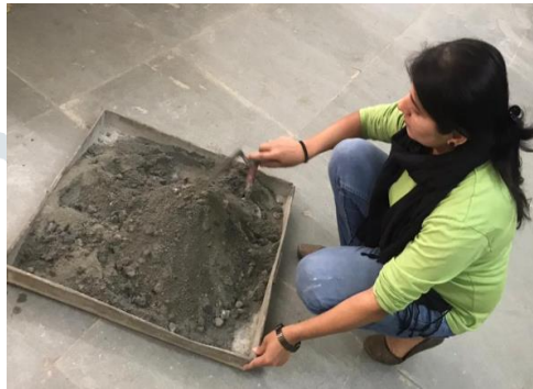
Fig.4.1 cement, jelly, M sand is taken in a tray and mixed properly
