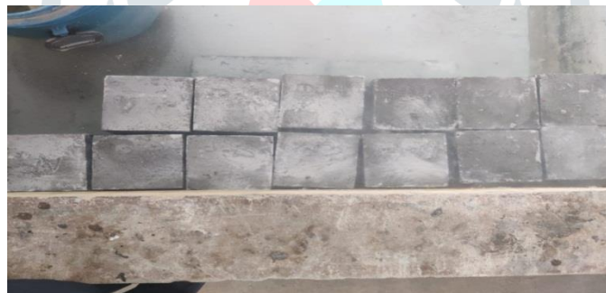
Fig 4.5 Curing process of the manufactured bricks
