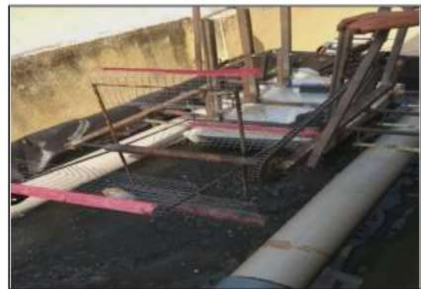
Fig. 6: Photograph of experimental setup of a River Debris Cleaning Machine
