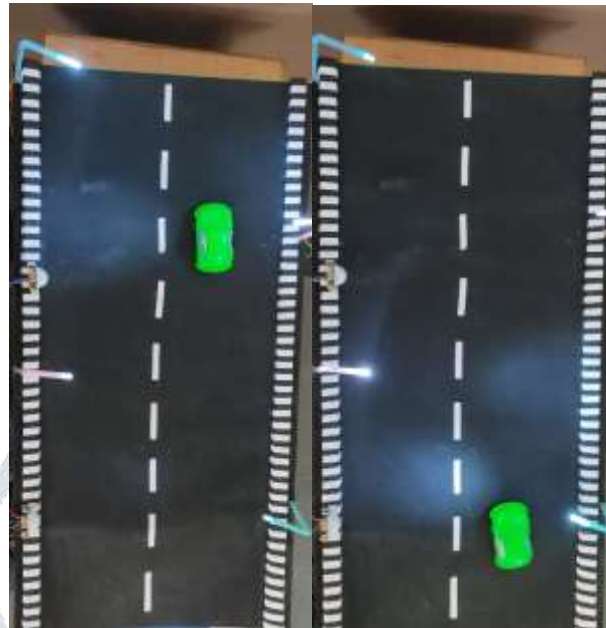
Figure 6. Switching the brightness of lights from 100% to 20% depending upon vehicle movements.
