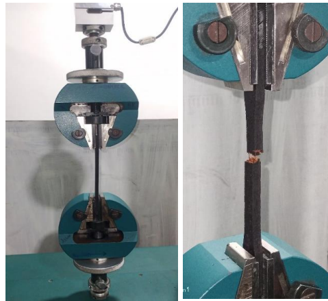
Figure 3.1: Test set up for tensile test
