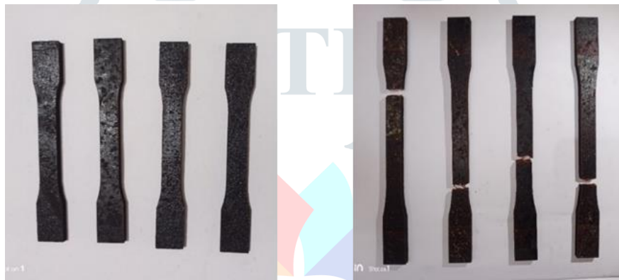
Figure 3.2: Test specimen before and after Tensile Test
