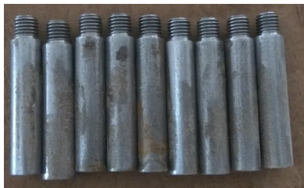
Figure 2: Piles of length 50 mm
