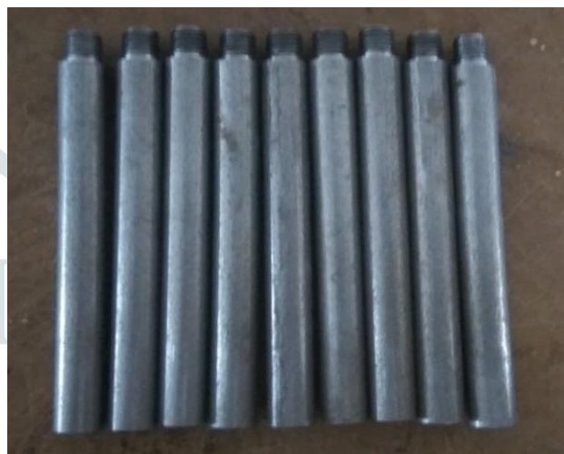
Figure 3: Piles of length 100 mm
