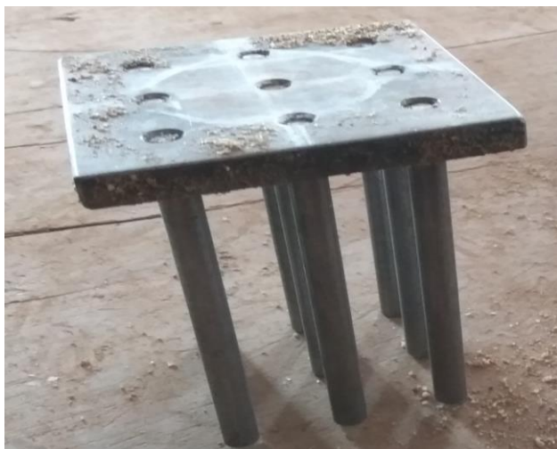
Figure 7: Fixing of nine piles to the raft
