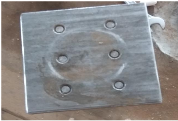
Figure 6: Fixing of six piles to the raft
