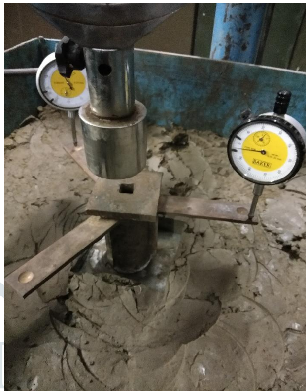
Figure 11: Testing model piled raft
