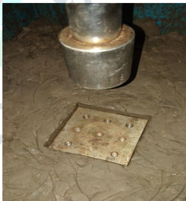
Figure 12: Uniform settlement is observed during the test.
