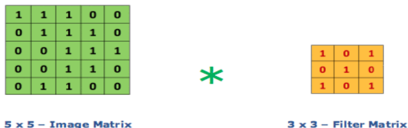
Fig 3.2.1 Input image 5 x5 convolve Operation with 3x3 filter matrix
