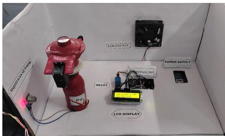
Hardware Implementation LPG Gas Accident Alert, Prevention
