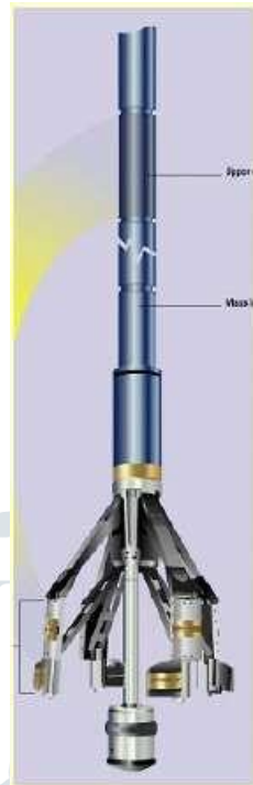
Fig: dipmeter logging tool
