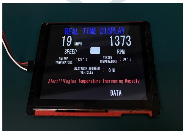
Fig. 8. Message (!!!Alert, Engine temperature increasing rapidly, slow down or stop the vehicle!!!)
