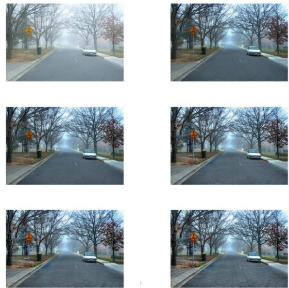
Figure 1.5: Influence of the clip-range parameter c . (a) Road Image (b)–(f) Result of dehazing with (b) c = 0.003 (c) c = 0.005 (d) c = 0.010 (e) c = 0.015 (f) c = 0.020 .
