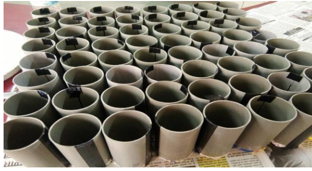
Figure 3.2 PVC cylindrical concrete moulds Cube: Concrete cube specimen of size 150mm x 150mm x150mm receptively.
