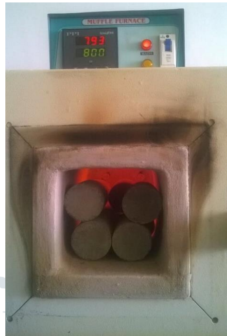
Figure 3.5 (a) Time-temperature curve for the center of the specimen and outer surface of the specimen (Lin et al. 2011); (b) Heating of the specimens at elevated temperature in electric muffle furnace.
