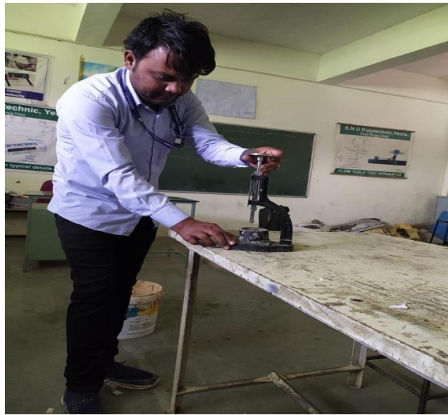
Photograph No. 3.1: Determination of Initial and Final setting time by Vicat apparatus
