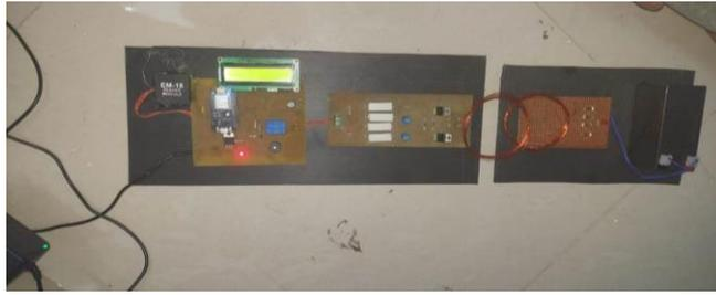
The simulation produced the anticipated outcomes, which are as follows: first, the car would arrive and then stand in a particular location with a primary coil at the bottom. Next, a person would scan an RFID card to complete the transaction, after which the vehicle would begin to charge. This information about the transaction, the charging location, the charging spot, the charging time, the charging cost, and all other related information would be recorded.
