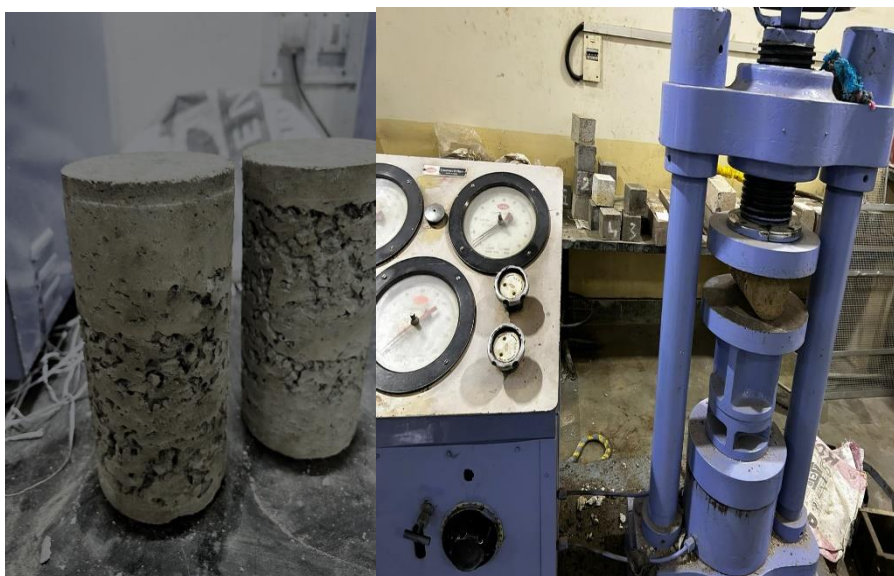
Fig 10 and 11: Cylinders cast for split tensile testing
