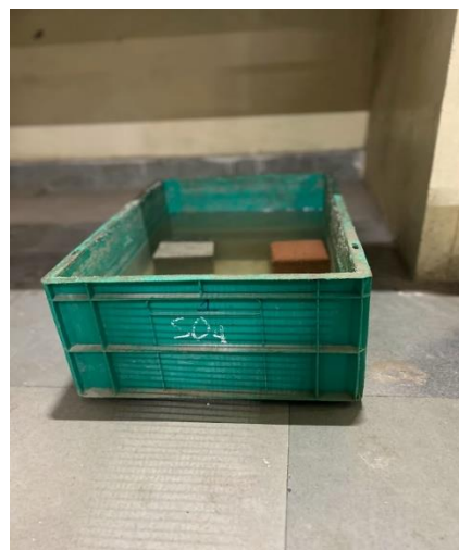
Fig 16: Specimens subjected to sulphate attack
