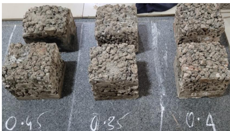
Fig 9: Cubes cast for optimum alkaline binder ratio
