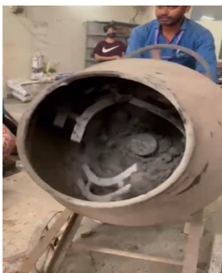
Fig 8: Manufacturing Fly ash aggregate in the laboratory
