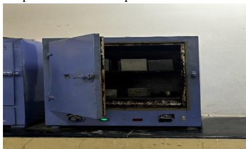
Fig 14: Cubes cast and cured in oven at different durations
