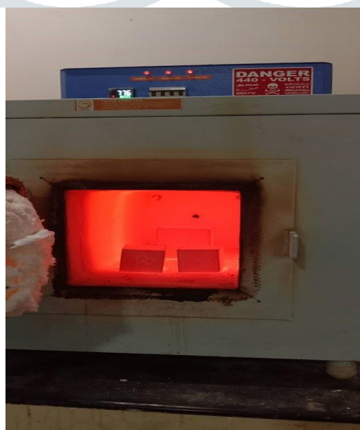
Fig 14: Cubes cast and subjected to higher temperatures
