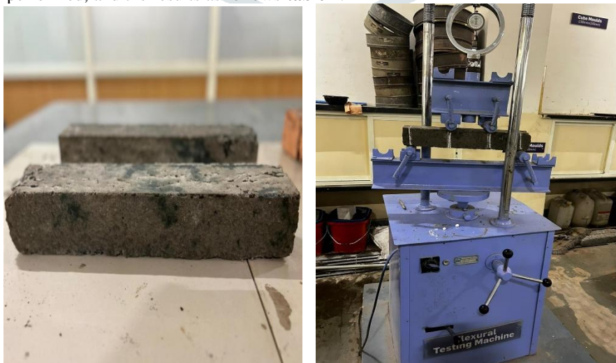
Fig 12 and 13: Prisms cast for split tensile test
