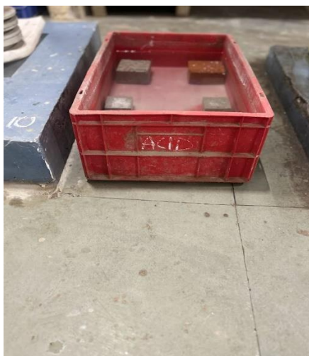
Fig 15: Specimens subjected to acid attack
