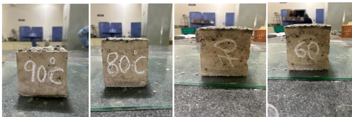
Fig 13: Cubes cast for determining the optimum curing temperature
