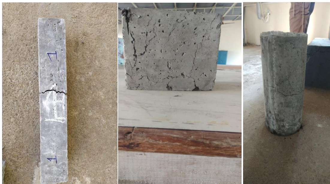
Fig 4.3.4 fractured concrete specimens
