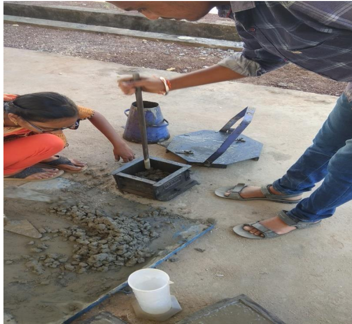
Fig 3.2.3 Placing and Compacting of Concrete in the Moulds
