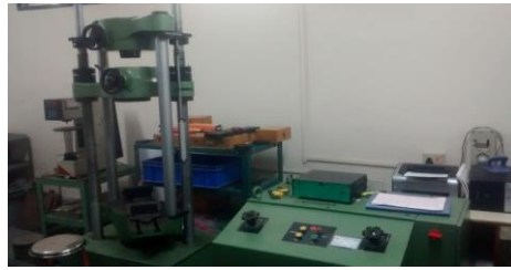
Fig.3.3.1 Photograph of Tensile Testing Machine
