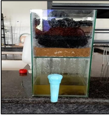
Figure 4.6 Filtration Media and its process
