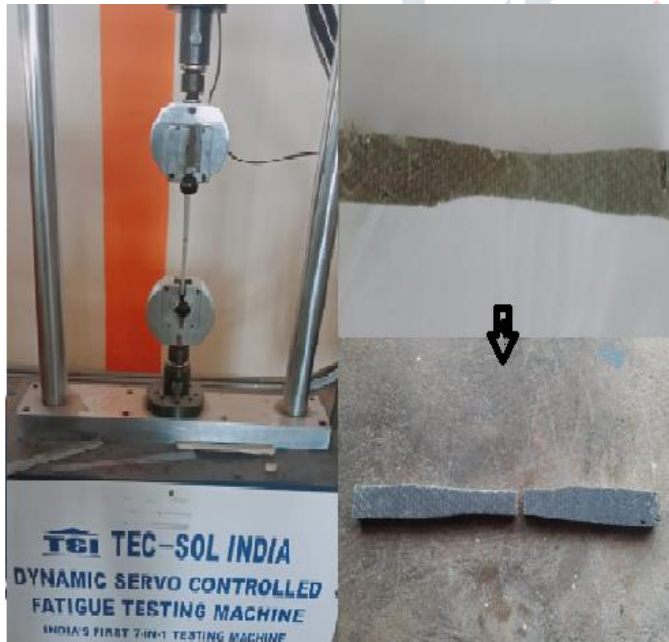
Fig .7 Tensile test occur in fatigue testing machine .
