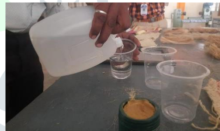
Fig 5. Mixing of resin
