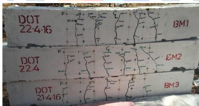
Figure -15: Deflected shape and Crack pattern of BM bacterial concrete beam specimens
