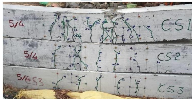
Figure -14: Deflected shape and Crack pattern of control concrete beam specimens
