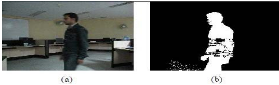
Diagram 3.2: Background Subtraction Results (a) Original picture (b) Picture after subtraction of background
