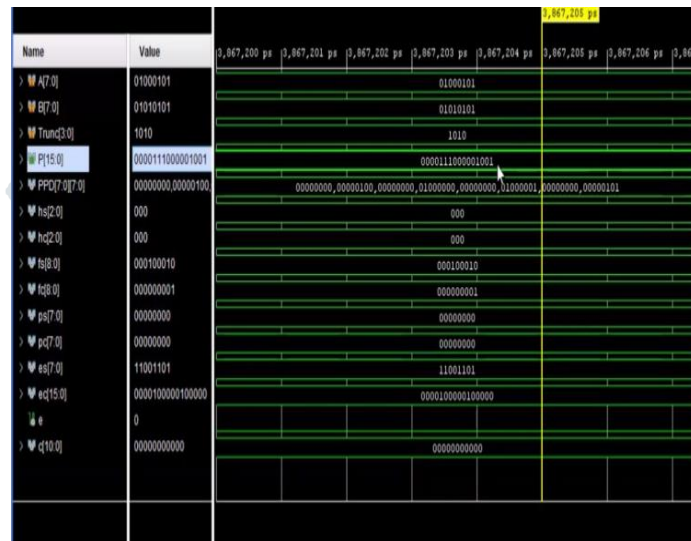
Figure 9: Output Waveform of Approximate Multiplier with 4-bit dynamic Truncation technique using approximate 4:2 compressor.
