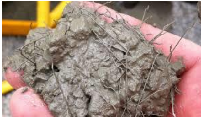
Fig.1. Steel Fiber Reinforced Concrete
