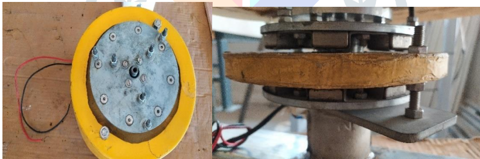
Fig3.Final assemble of generator
