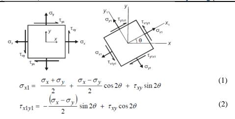
These equations 1 and 2 can be used to calculate a new set of values  $\sigma_{x1}$ ,  $\sigma_{y1}$ , and  $\tau_{x1y1}$  for any new position of the axes for various values of  $\theta$  ranging from  $0^{\circ}$  to  $180^{\circ}$ . The values are repeated from  $180^{\circ}$  to  $360^{\circ}$  due to the symmetry of the equations. Equations involve the expression  $2\theta$  which implies that the values are repeated every  $180^{\circ}$ .
