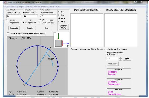
Pressing the "Details" button gives the following screen which presents details pertaining to principal stresses, maximum shear stress and their inclinations.
