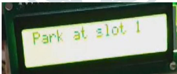
Fig 5: Lcd Showing parking Allotment
