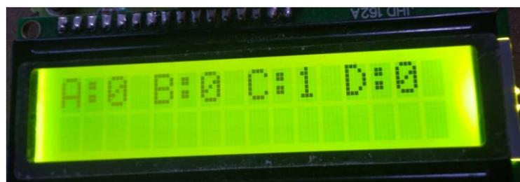
Fig 6: LCD showing Slots Status
