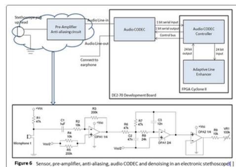
Figure 6 Sensor, pre-amplifier, anti-aliasing, audio CODEC and denoising in an electronic stethoscope [ ]
