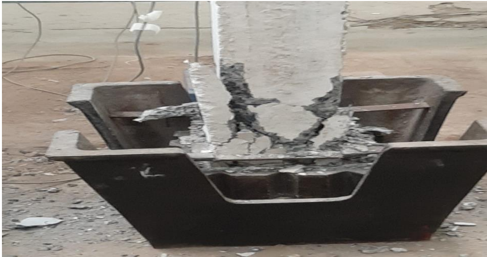
Fig 5.0: Column with 10mm steel as longitudinal rebar's. SPECIMEN 1
