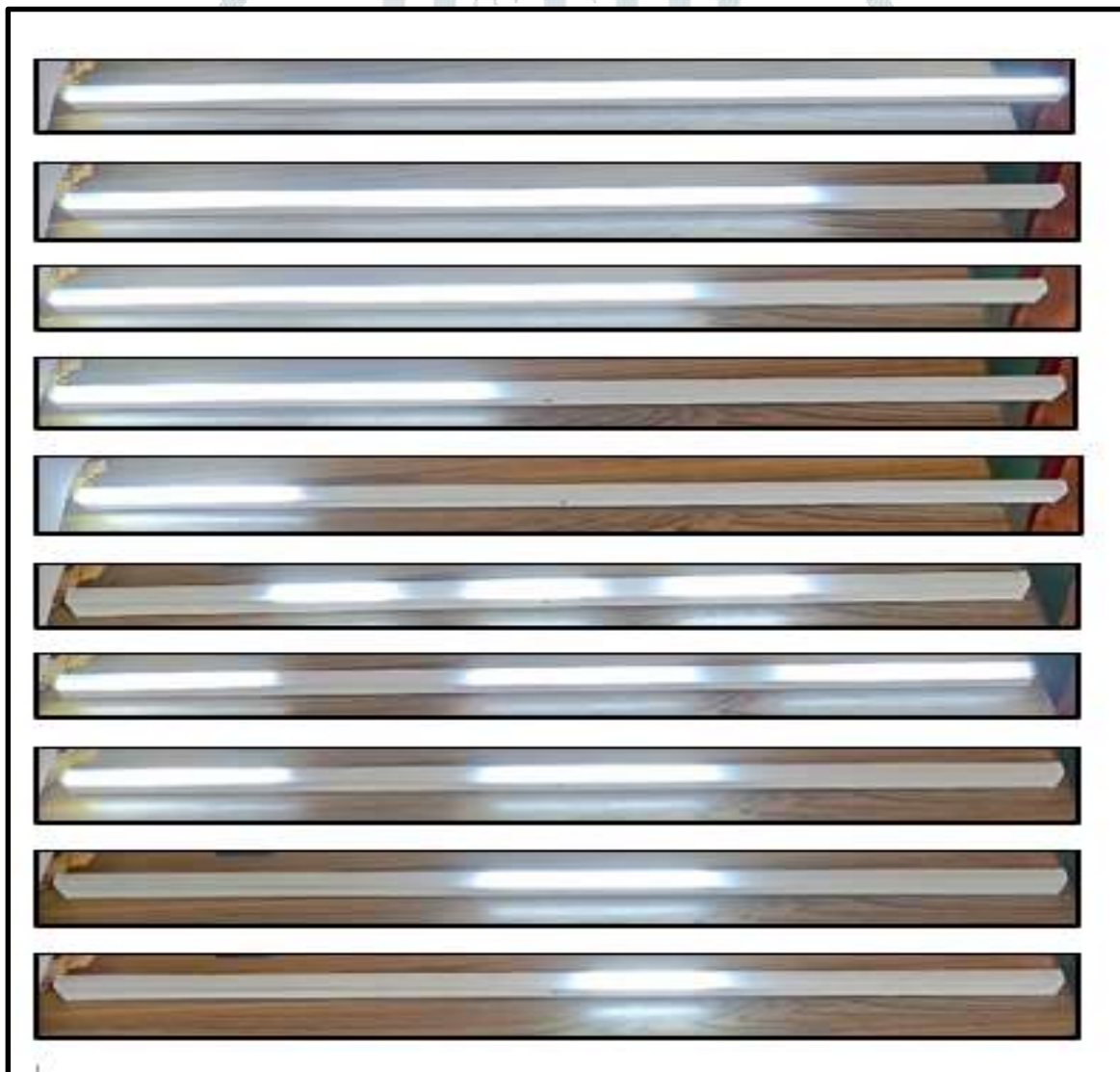
Figure 11: Lighting Pattern Under Various Segment Activations
