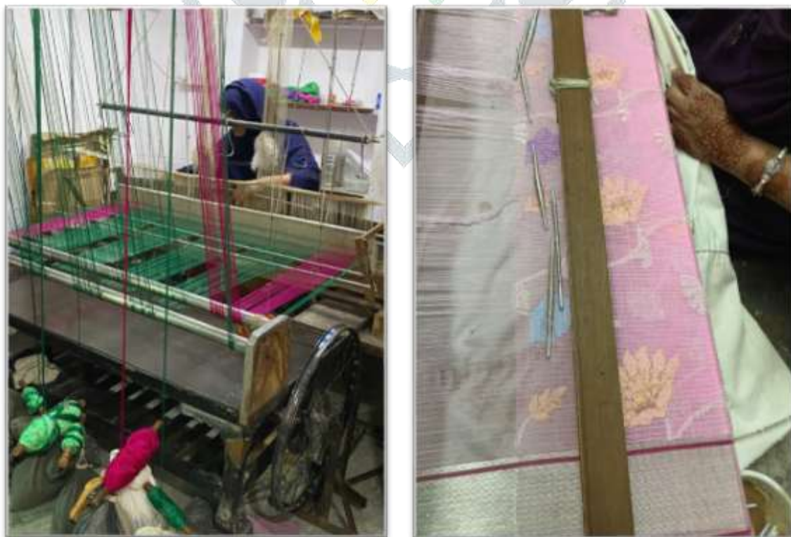
Figure 2: Female weaver interlacing cotton and silk threads on a Kota Doria handloom (Photo by author, 2024)
